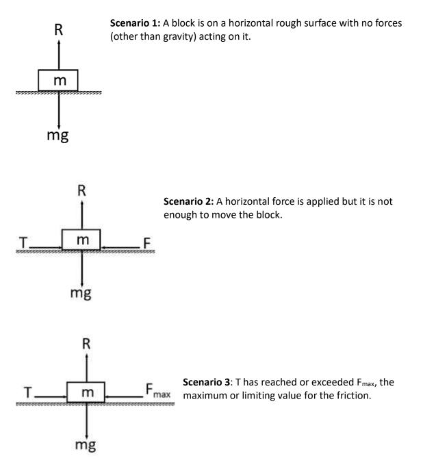
Two things determine the maximum or limiting value,  $F_{max}$  between two surfaces:
